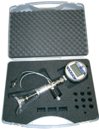
Basic version incl. pneumatic pressure generation
